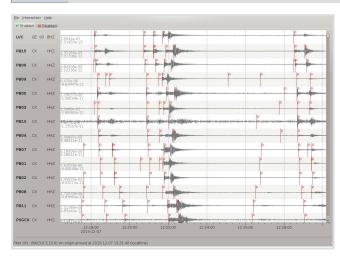
**scanloc** is a clustering and association tool to detect and to locate local to regional earthquakes using the cluster search algorithm DBSCAN. The cluster search in scanloc identifies phase picks from a cloud of possible picks reliably associating them to earthquakes. It also associates additionally incoming P- and S-phases to already existing internal or external hypocentre solutions.
