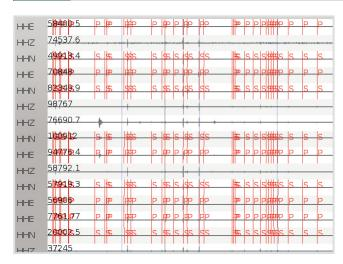
**ccloc** detects earthquakes and other seismic events at very low to large magnitudes by matching waveform templates from known master events to real-time or archived data. Computing on GPU is applied for highest performance.
